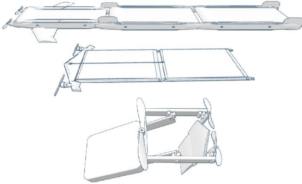
**Figure 1.** Transformer and SP-Drone configurations with one towed platform.
