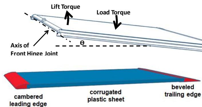
**Figure 2.** Side view of flat plate part of flat plate airfoil illustrating variables and axis of analysis.
