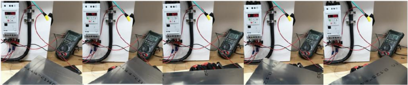
Figure 1. Picture sequence of rotating (2' X 2' X 1/8") sheet of aluminum over three coils of linear motor. The sheet undergoes magnetic suspension force and clockwise (left to right) propulsion force. The frequency (Hz) and voltage are displayed on meters as the Eaton controller ramps up in frequency. The sequential voltage values are 10, 25, 37, 48, and 61 V with rotation rate increasing rapidly in this 5-second sequence.
