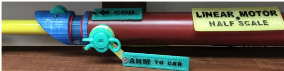
Figure 2. 3D print of half-scale linear motor stator (burgundy and blue) over tube armature (yellow). In today's R&D approaches, the gap between printing of 3D representations and working prototypes is becoming increasingly small.
