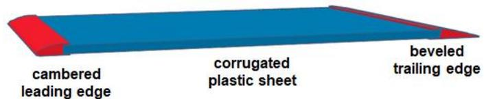
**Figure 11.** Side cross section of practical flat plate airfoil.
