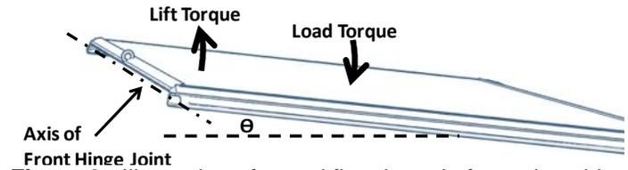
**Figure 9.** Illustration of towed flat plate platform pivotable about a front hinge joint.
