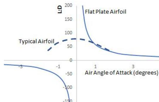
**Figure 10.** L:D of flat plate airfoil and a typical wing airfoil.
